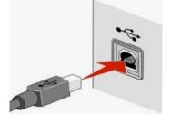
how to connect the standard USB male connector to our computer, but there is more confusion with the other end of that USB cable that attaches into (usually) the back of the printer (see the picture to the right).
